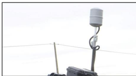
External dome antenna on a motorcycle or under a helicopter
